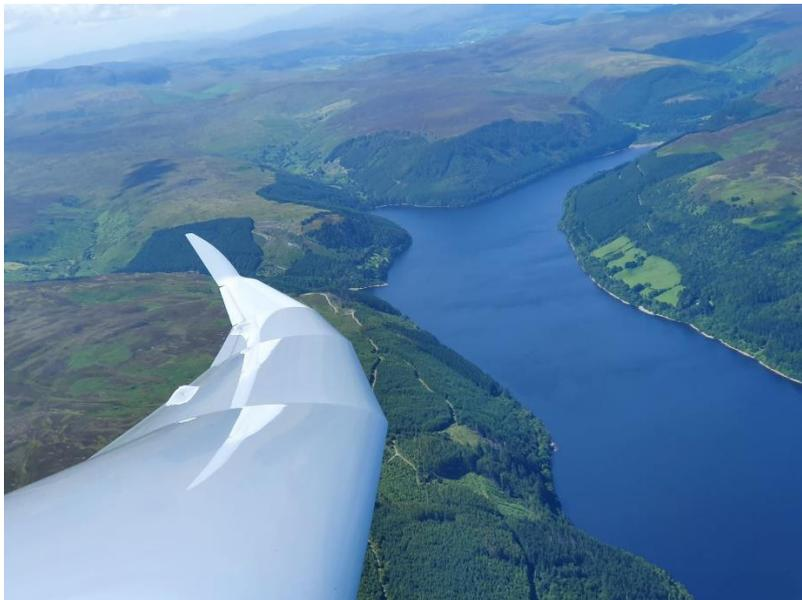
The glider I fly has a wingspan (wing tip to wing tip) of 20 metres which roughly equates to about one and a half shortmats laid end to end. It is made of carbon fibre covered in a coat of acrylic which is polished to maintain a smooth surface to maximise the airflow. Another flight on Tuesday was a 500km (310 miles) flight along the south coast and back in just 5 hours flying time, using only the power of the sun to create thermals and a bit of skill in finding them.
